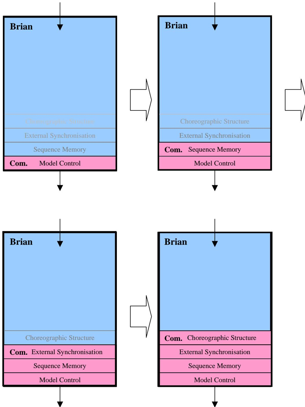
**Diagram 3** – Software Developmental Process Showing Transference of Functionality from Operator/Programmer (Brian) to the Computer
